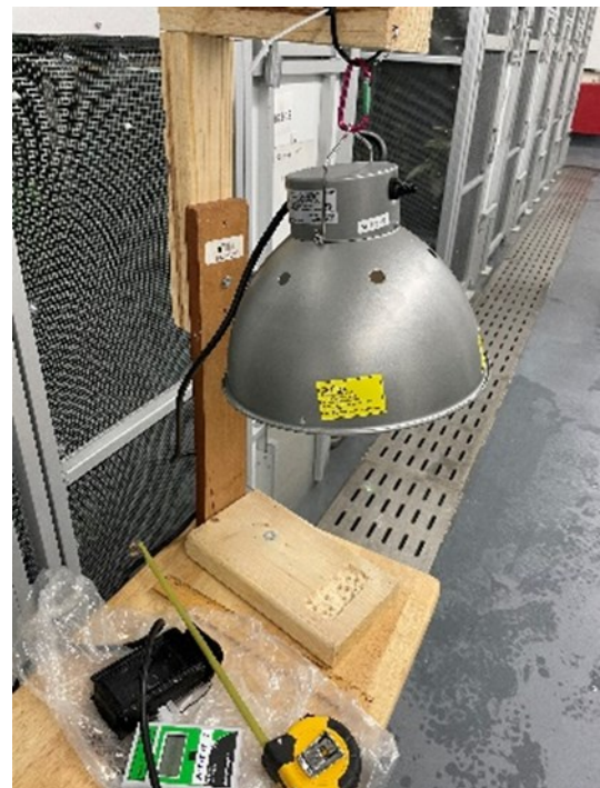
UV bulb testing stand built to hold bulbs at 30cm above the meter to standardize measurements.
