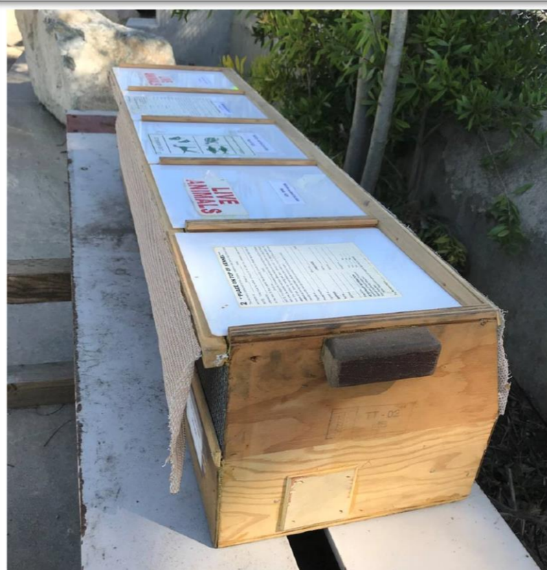
Broad details of shipping design: flow through ventilation, opaque top, mosquito netting under hardware cloth, light color shade cloth for privacy but still allow maximum light
